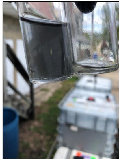
Photo 4: View looking north. PlumeStop qualitative concentration test showing influence in MW-24. (Apr 27, 2020).
