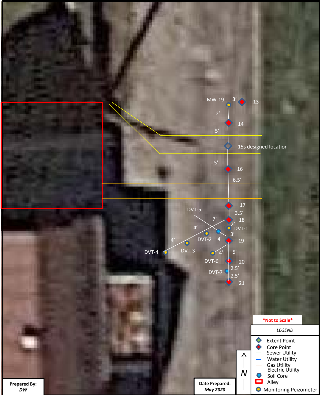
Figure 1 – Barrier C DVT Location Map O’Neals Clothes Depot Cleaners 833 East Morgan Street Martinsville, IN
