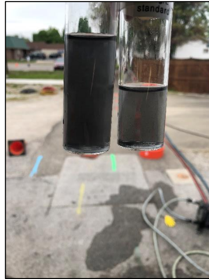
Photo 10: View looking east. PlumeStop qualitative concentration test showing influence in MW-8. (May 13, 2020).
