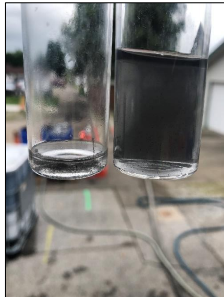
Photo 12: View looking east. PlumeStop qualitative concentration test showing influence in MW-9. (May 21, 2020).
