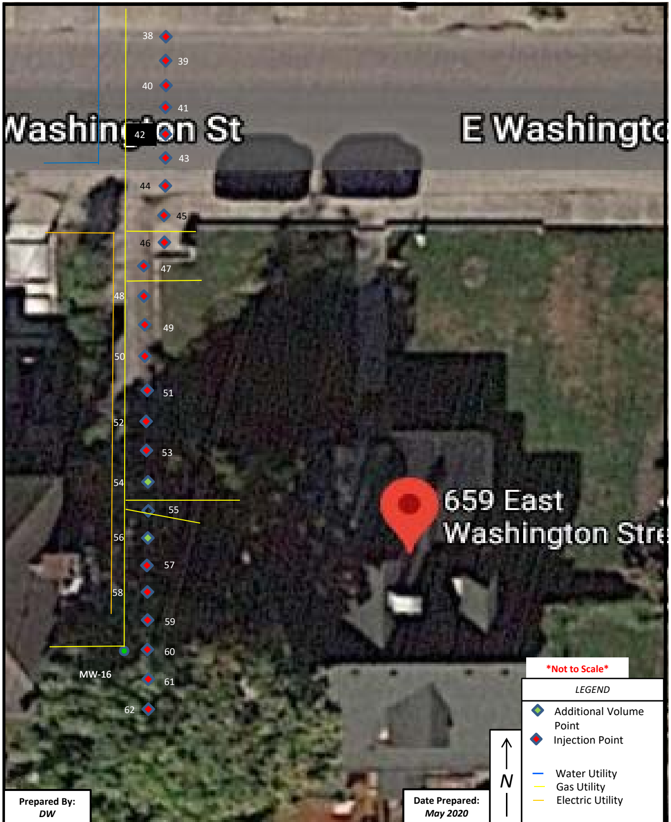
Figure 4 – Barrier B N-S Locations Map O’Neals Clothes Depot Cleaners 833 East Morgan Street Martinsville, IN
