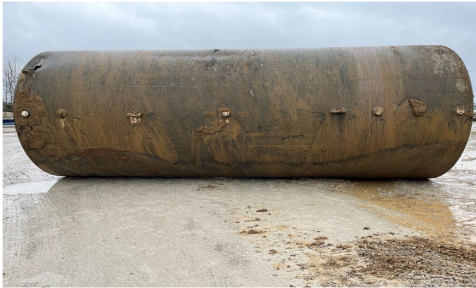
Photo 1 – 15,000-Gallon UST post excavation
