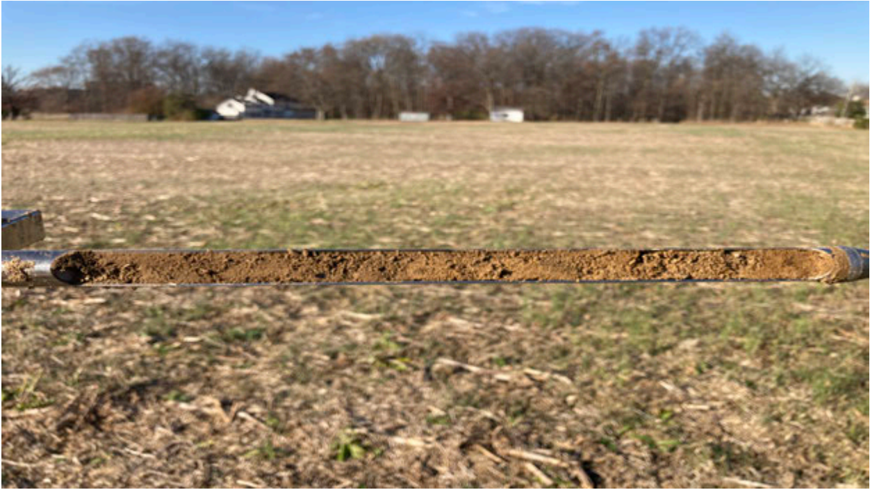
Photos 2. Typical soil profile of Miami silt loam (MmB2), taken at Sampling Point # 1.
