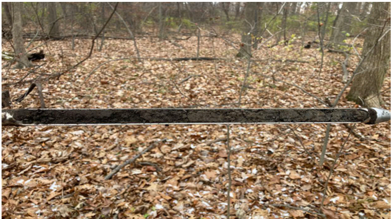
Photo 10. Typical soil profile of Brookston silty clay loam (Br), taken at Sampling Point # 7.
