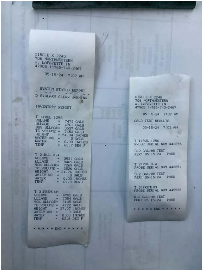
Monthly Inspection Checklist -> Release Detection -> Automatic Tank Gauge (ATG) - Passing tank test results
