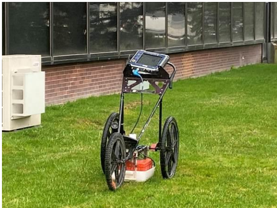
Photo #3: View of utility locating equipment (4/6/2022).
