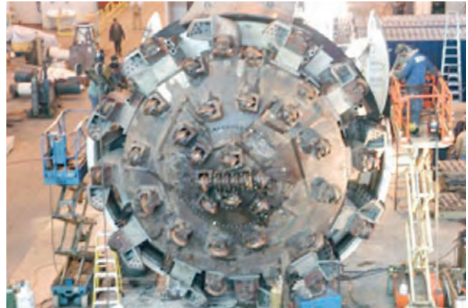
A typical rock tunnel boring machine is shown in the photo.
