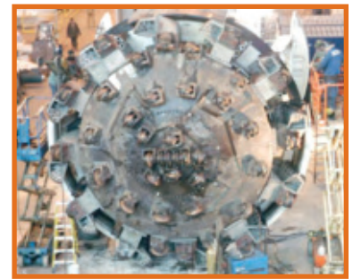
The photo above shows a typical cutter head on a rock tunnel boring machine. The machine will bore through the limestone bedrock more than 200 feet below ground level, cutting a tunnel 7.5 - 10 miles long and 26-35 feet in diameter. Construction is still several years away.
