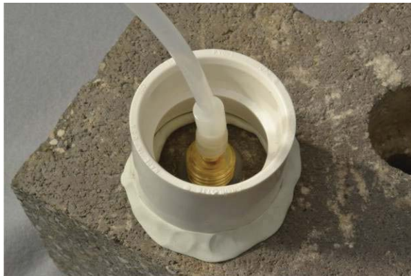
Figure 6. Water dam used for leak detection.
