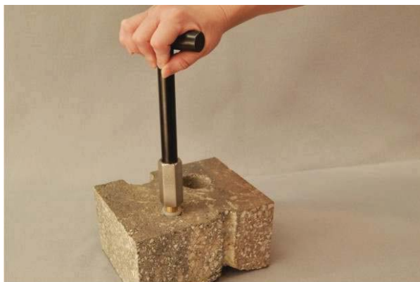
Figure 7. Removing the Vapor Pin™.
