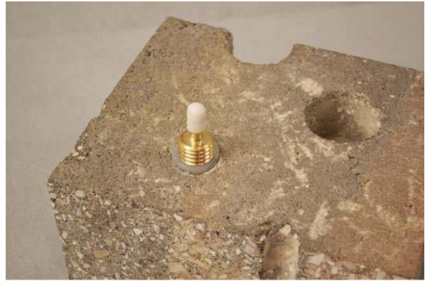
Figure 4. Installed Vapor Pin™.
