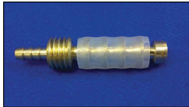
Figure 1. Assembled Vapor Pin™.
