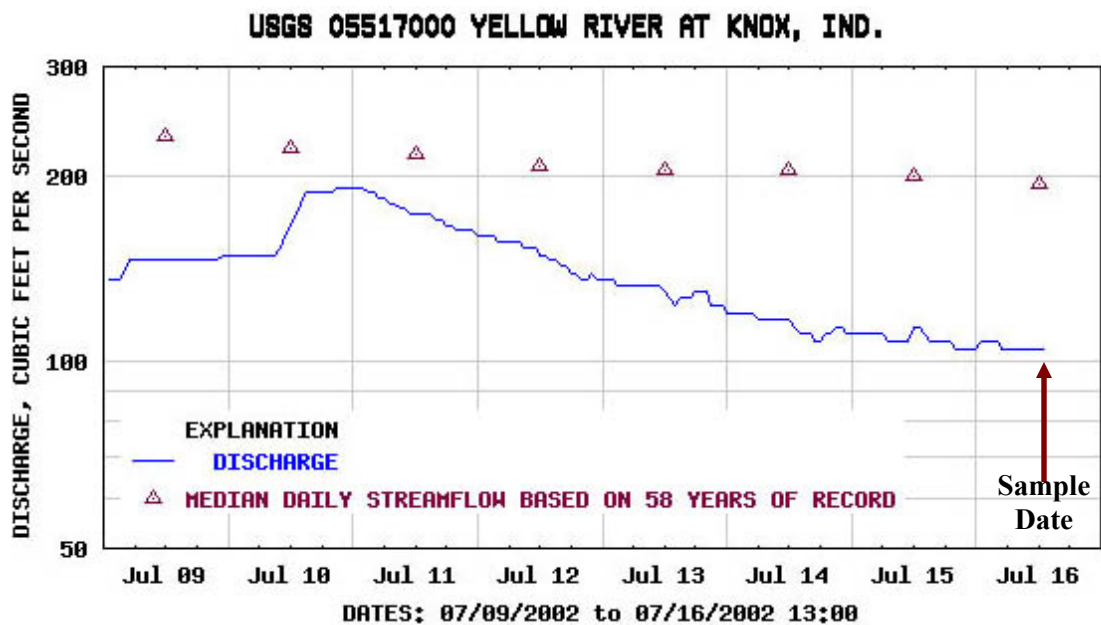
Figure C. Mean daily discharge for the Yellow River at Knox, Indiana with base flow sampling date noted. Discharge on the sampling date was well below the 58-year median stream flow.
