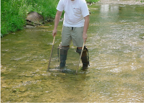
Figure 3-2: Demonstration of Kick Seine Sampling Method
