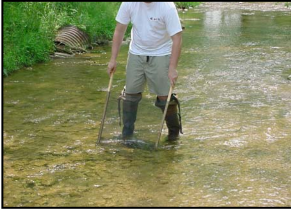
Figure 3-2: Demonstration of Kick Seine Sampling Method
