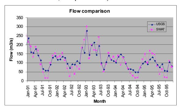
Figure 2: SWAT monthly flow and USGS gage station data comparison near Niles, MI (USGS Station No. 04101500) for the period of January 1991 to December 1995.
