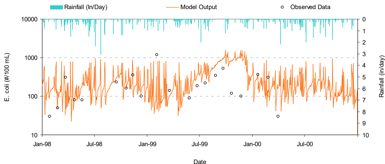
Figure 20. Comparison of modeled to observed predicted E. coli at station WWU010-0001 (east edge of Muncie) for the period January 1, 1998, to December 31, 2000.
