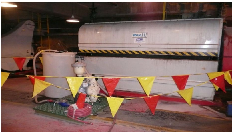
Photo 1. Entrainment setup following Traveling Screens at Lakeside Pump Station
