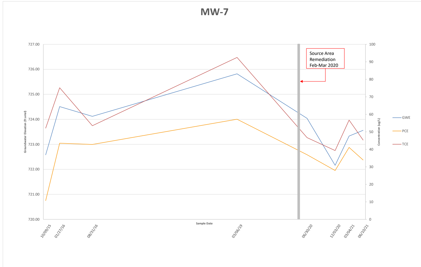
Figure 4 PCE and TCE Concentration Trends with Groundwater Elevations Reed Manufacturing Services Franklin, Indiana IDEM State Cleanup # 2013-42015
