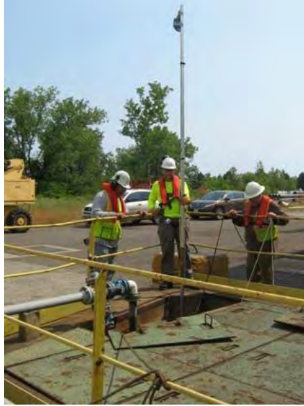
Photo 4. Photograph showing the DIDSON deployed in the pre-well at the Midwest CWIS in June, 2012.
