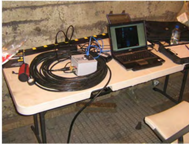
Photo 1. Photograph showing the topside components of the DIDSON data collection system used during Phase 1 of the 316(b) Special Studies conducted at Midwest CWIS in 2012 through 2014.
