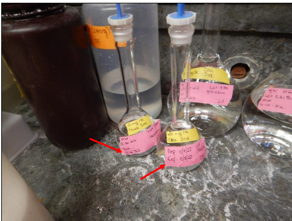
Photograph 40. Onsite Laboratory – View of ammonia analysis reagents with expiration dates two to three weeks prior to the date of the inspection (October 27, 2022). Laboratory representatives stated new reagents would be mixed prior to the next analysis.
