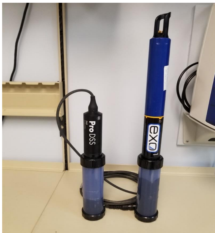
Figure 4. Image of a ProDSS sonde with cable assembly and calibration cup attached and an EXO sonde with calibration cup attached.
