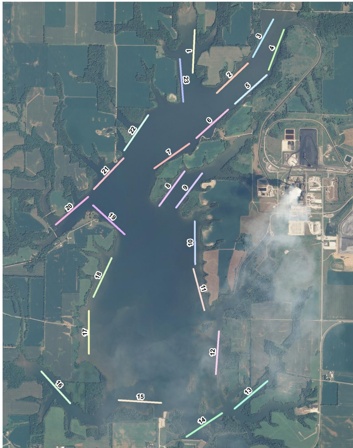
Figure 1 Example of a waterbody shoreline divided into 500-meter stations for fish community sampling
